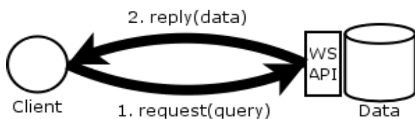
Figure 1. A traditional pull-based client-server architecture.
